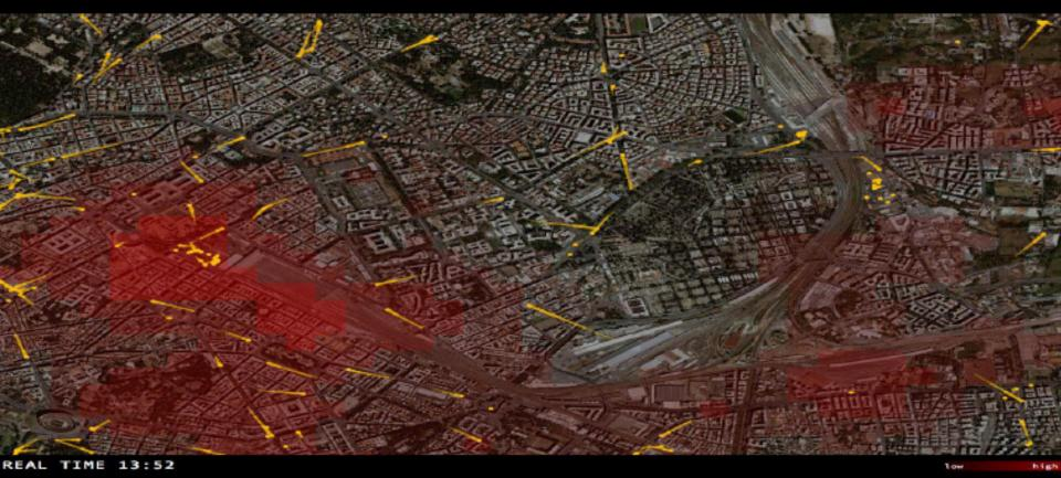
It shows the changing positions of Atac buses, indicated by yellow points, and the relative densities of mobile phone users, represented by the red areas. If a tail on a yellow point is long, that means that a bus is moving fast. Areas colored by a deeper red, have a higher density of pedestrians
